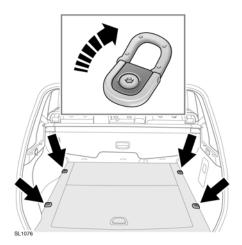
To assist in safely securing large items of luggage, four fixing points are located in the rear loadspace floor.
