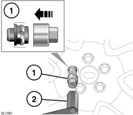
1. Insert the wheel nut adapter into the locking wheel nut, ensuring that it is fully engaged.
