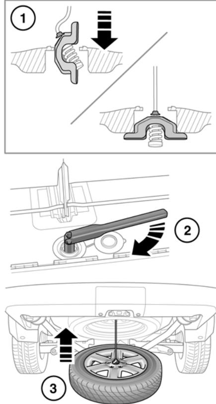
**WARNING:** Do not stow the wheel while the vehicle is raised on the jack.
