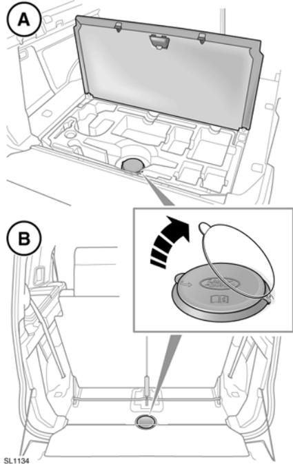
**WARNING:** Remove the spare wheel prior to jacking the vehicle, to avoid destabilizing the vehicle when raised.
