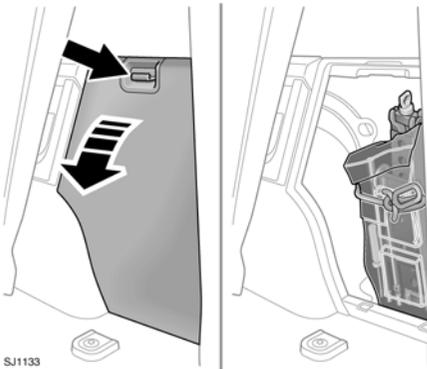
**7-seat vehicles:** The tool kit is stowed behind an access cover in the loadspace area.
