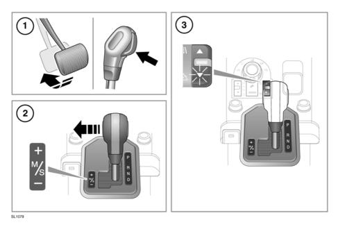
1. To select Drive (**D**) when the vehicle is stationary, apply the foot brake and press the gear selector release button.
