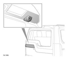
When reverse gear is selected, the screen automatically displays a wide angle, color image from the rear of your vehicle.
