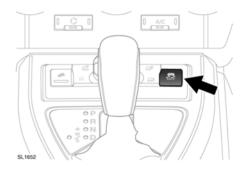
To disable DSC, press and briefly hold the DSC OFF switch on the fascia (the DSC off warning lamp
