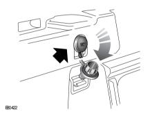
On 7-seat vehicles, a third power socket is fitted in the left-hand side trim in the loadspace area.
