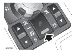
Press and release the switch (arrowed) to select HDC, the HDC information indicator will illuminate. To deselect, press and release the switch again (indicator extinguishes).
