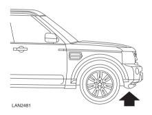
When the heater is operating, exhaust fumes from the heater may be seen coming from underside the vehicle. This is normal, and is not a cause for concern.
