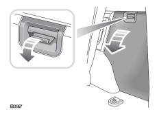
There are access hatches on both sides of the rear loadspace.
