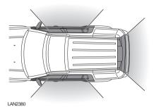
Keyless entry allows the driver to unlock and disarm the vehicle by simply operating the door handle. The Keyless Entry function operates in the following manner:
