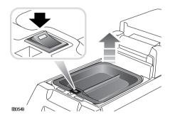
The cool box is switched on/off using the switch on the inside front lip of the cool box. There is a short delay between pressing the switch, and illumination of the indicator.
