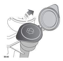
The washer reservoir supplies both front and rear screen washer jets and headlamp washer jets.
