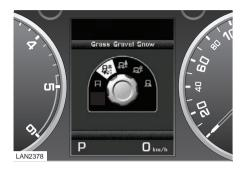
The temperature and fuel gauges will be temporarily replaced on the message centre with a representation of the Terrain Response control. The current active program is shown as a white icon on a black background.
