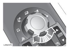
With the ignition switched on, one of the indicators around the control will illuminate amber to indicate the currently selected active program. The special program indicator will also be displayed on the message centre.
