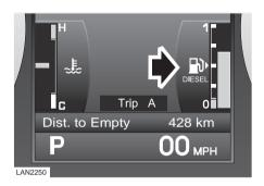
When the ignition is switched on, the gauge quickly rises to show the level of fuel in the tank.
