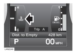
If the indicator moves above the mid point, the engine coolant is becoming too hot. If the indicator moves into the **H** segment at the top of the gauge severe engine damage could occur (under these circumstances the air conditioning may switch off and engine performance may reduce to minimise engine load).
