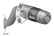
Turn the wiper switch to position **1.** The wipers will operate for a single wipe and then the interval between subsequent wipes is controlled by the rain sensor.
