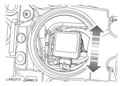
**Note:** On LHD vehicles fitted with halogen headlamps, the lever is on the left-hand side of the bulb aperture.
