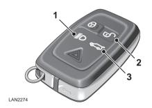
To raise the suspension, press and hold button and button 2.
