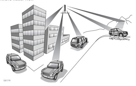
Some interference is to be expected from time to time during a journey. Occasionally, it may be necessary to retune the audio unit, to offset the effects of moving from one transmitter area to another.
