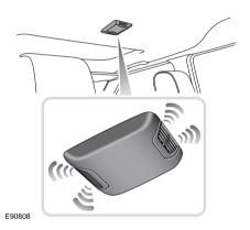
Roof-mounted intrusion sensors monitor the interior space and activate the alarm if movement of air is detected in the passenger compartment.
