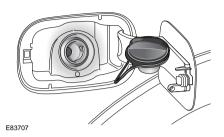
The filler cap is secured to the vehicle by a strap, and a holder is provided on the flap to locate the cap during refuelling.
