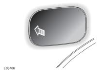
With the vehicle unlocked using the Smart Key. press and release the centre of the left edge of the fuel filler flap (where arrowed) to open.
