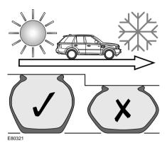
If the ambient temperature drops, the tyre pressures will decrease, which may cause under inflation. This may happen when travelling to, or through, areas of significantly lower temperature.
