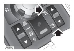
The transfer gearbox allows selection of high or low range gears.
