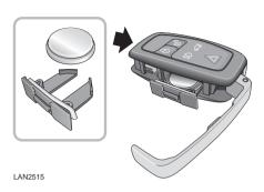
When the battery needs renewing, there will be a significant decrease in the effective range of the Smart Key transmitter and the message **SMART KEY BATTERY LOW** is displayed in the message centre.
