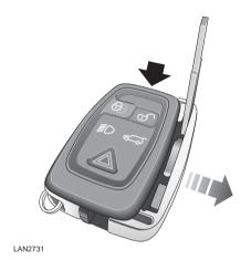
**To extract:** Press and hold the release button, pull out the key blade compartment to expose the key.
