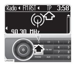
Normal reception can be interrupted to broadcast traffic information from stations on the FM waveband or Radio Data System (RDS) and Enhanced Other Network (EON) linked stations.
