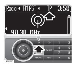
Normal reception can be interrupted to broadcast traffic information from stations on the FM waveband or Radio Data System (RDS) and Enhanced Other Network (EON) linked stations.
