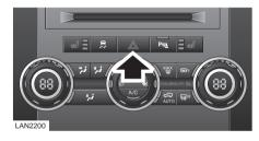
Press the switch to operate the hazard warning lamps. All of the direction indicator lamps will flash together.
