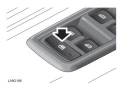
To prevent operation of the rear window switches, press the isolator switch. Press the switch again to restore independent control.
