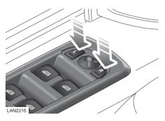
To fold the mirrors, press both the L and R mirror switches at the same time. To unfold the mirrors, press both of the switches again.
