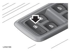
To prevent operation of the rear window switches, press the isolator switch. Press the switch again to restore independent control.
