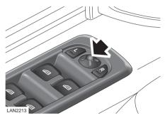
Press the L or **R** switch to select the required mirror. The tell-tale light in the switch will illuminate to indicate that it has been selected.
