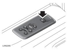
The rear windows can be operated from the switches on the rear doors if the rear window isolation switch has not been activated.
