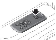
The rear windows can be operated from the switches on the rear doors if the rear window isolation switch has not been activated.
