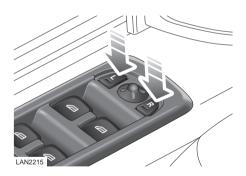
To fold the mirrors, press both the  ${\bf L}$  and  ${\bf R}$  mirror switches at the same time. To unfold the mirrors, press both of the switches again.
