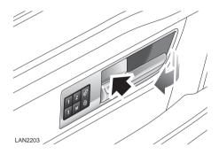
From inside the vehicle, all the doors can locked by pressing either the driver or passenger lock lever (arrowed).
