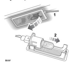
Follow the steps illustrated. Insert a new bulb and refit the components.
