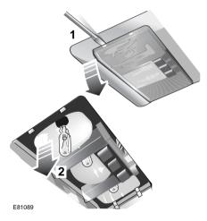
Follow the steps illustrated. Insert a new bulb and refit the components.
