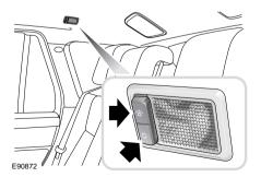
Press the switch on the lamp to operate.
