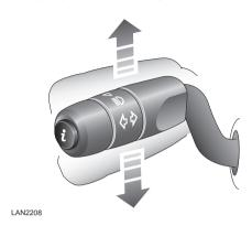
With the ignition switched on, move the lever up or down to operate the direction indicators.
