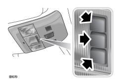
Each lamp can be switched on or off by pressing the switch adjacent to the lamp required.
