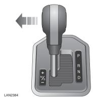
To select Sport mode, move the gear lever from the **D** position towards the left hand side of the vehicle. **S** will appear in the gear selector display and the LED to the side of the selector lever illuminates.
