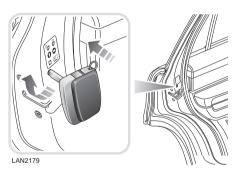
Child safety locks are fitted to the rear doors. Insert the starter key into the keyhole and turn outwards to activate the child safety lock.
