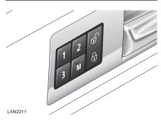
The vehicle can memorise up to three different driver seat, exterior mirrors and steering column positions. This enables three different drivers to achieve optimum comfort at the touch of a button.
