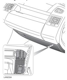
The passenger compartment fuse box is fitted behind the glove box. To access the fuses, open the glove box and then pinch the top of the support stays, and lower the glove box into the footwell.
