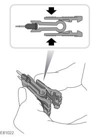
The fuse removal tweezers are located in the passenger compartment fuse box. Place the tweezers onto the head of the suspect fuse (as shown), squeeze the middle (arrowed) and pull to remove. A break in the wire inside the fuse indicates that the fuse has blown.
