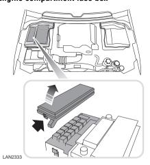
Remove the plastic cover by pressing the tabs. The fuse values and locations and the circuits protected are shown on the plastic cover.
