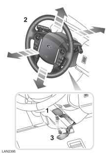
The steering column position can be adjusted in two directions.
