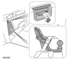
The tow ball is stowed under an access cover in the loadspace floor (5-seat models) or behind an access cover on the left-hand side of the loadspace (7-seat models).
