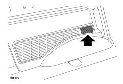
A fixed vent on the left-hand side rear quarter panel provides airflow to the third-row seat lower area.
