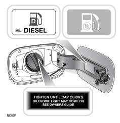
The correct fuel specification for your vehicle is shown on the inside of the fuel filler flap.
