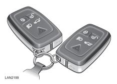
The security system and entry to the vehicle are controlled by the Smart Key remote control. All doors and the luggage compartment can be locked and unlocked using the remote control buttons.
