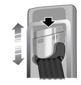
Press down (solid arrow) to release the catch, then lift or push down to adjust the height of the anchorage.
