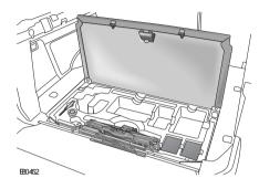
On 5-seat vehicles, the tool kit is located under a panel set in the loadspace floor.
