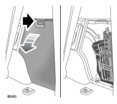
On 7-seat vehicles, the tool kit is stowed behind an access cover in the loadspace area.
