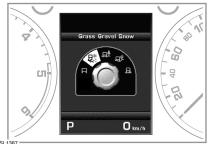
A rotary control just in front of the gear lever is used to select the required special program.
