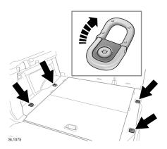
To assist in safely securing large items of luggage, four fixing points are located in the rear loadspace floor.
