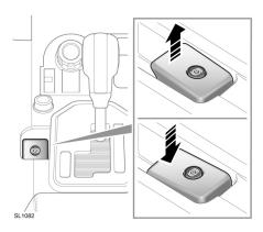
With the vehicle stationary, pull up the lever (arrowed) and release it.
