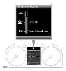
An indication of the oil level is displayed in the gauge. Messages to the right of the gauge advise you of any action you may need to take. If the oil level is within the required operating range, the message **Engine Oil Level OK** will be displayed. Do not add any additional oil to the engine.
