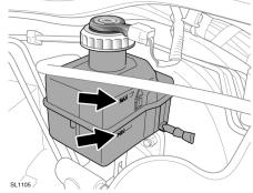
The left hand or right hand under bonnet cover must be removed to check the brake fluid level, dependent on the vehicle being left-hand drive (left hand cover) or right-hand drive. See 186, UNDER BONNET COVERS - REMOVAL.
