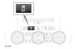
To disable DSC, press and briefly hold the DSC OFF switch on the fascia (the DSC off warning lamp will illuminate continuously). Deactivating DSC also reduces the level of Traction control intervention and may lead to an increase in wheel spin.
