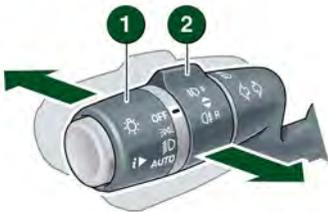
1. **Outer collar:** First position for side lamps, second position for headlamps and the third position for **AUTO**. With **AUTO** selected, all exterior lamps will switch on automatically when the ambient light fades.
