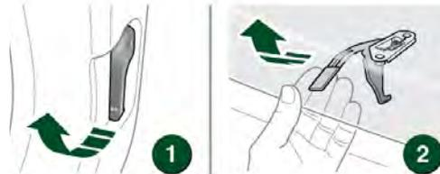
1. Pull the bonnet release lever, located in the left side front footwell.
