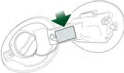
Twist the cap counter-clockwise to release. Replace the cap and turn it clockwise until the ratchet clicks. Close the fuel filler flap until it is latched in the closed position.
