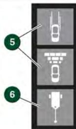
6. Hitch guidance: To aid the process of guiding the vehicle to the trailer's tow hitch. A single hitch line is displayed as the reversing guidance line. As the vehicle closes to within 0.6 m of the tow hitch, an automated zoom is operated.
