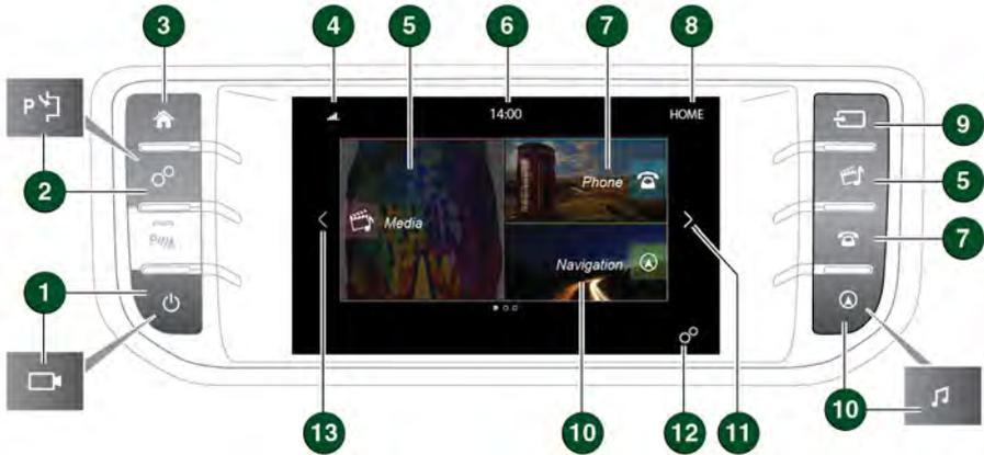
1. Press to switch the Touch screen on/off. If Surround cameras are fitted, the screen can be switched off in Extra features.
