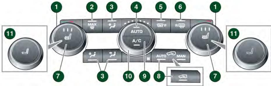
1. Temperature controls: Rotate to adjust the temperature.
