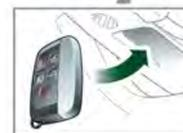
If, after closing all of the doors, the Smart key is not detected by the vehicle, **Smart Key Not Recognised - Place As Shown And Press Start Button** is displayed in the Message centre. With the brake pedal (automatic transmission), or clutch pedal (manual transmission), firmly pressed, press and release the **START/STOP** button. The Smart key can now be removed.
