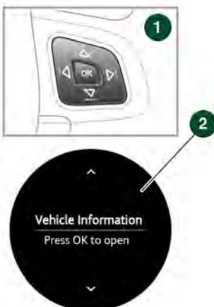
1. Steering wheel control: Use to scroll up or down through the menu to the feature you want to disable/enable.
