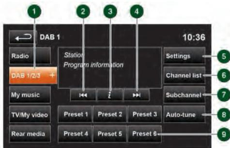
1. Touch to view and select a **DAB** band (**DAB 1**, **2** or **3**). The radio tunes to the last used channel on that band. Touch again to close.
