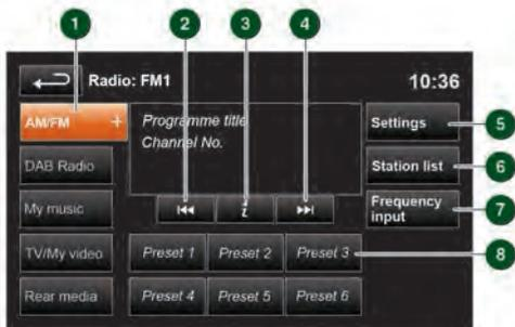
1. Touch to view and select wavebands. The radio tunes to the last used channel on that band. Touch again to close.
