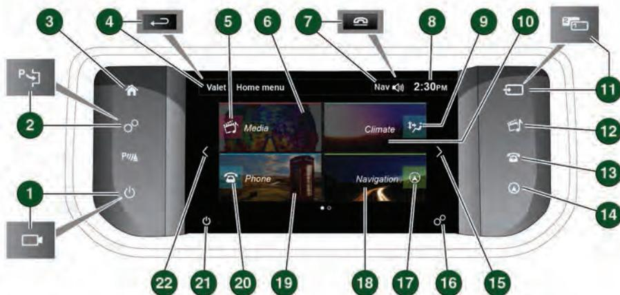
1. Press to switch the screen on/off. If Surround cameras are fitted, press to access the special views page.
