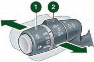
**1. Outer collar.** Rotate to first position for side lamps, second position for headlamps, third position for **AUTO**. With **AUTO** selected, all exterior lamps will switch on automatically when ambient light fades.
