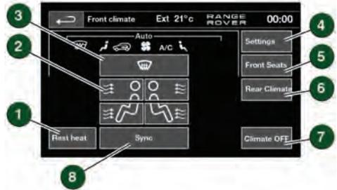
1. With the engine switched off, press to operate Rest heat. Uses the residual engine heat to provide cabin heating.
