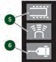
6. Hitch guidance. To aid the process of guiding the vehicle to the trailer tow hitch. A single hitch line is displayed as the reversing guideline. As the vehicle closes to within 0.6 m of the tow hitch, an automated zoom is operated.
