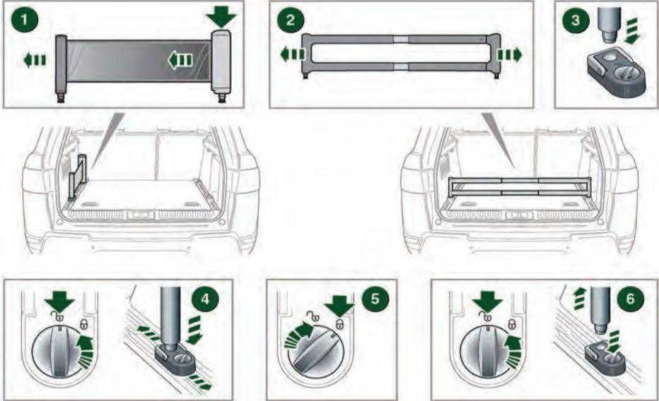
1. Press and hold while pulling out the luggage retaining band and adjust to the required length.
