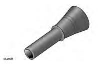
If the vehicle runs out of fuel and is fitted with an active misfuelling device, use the emergency funnel supplied with the vehicle, to refill the tank. This will open the misfuelling device to enable a fuel can to be used.
