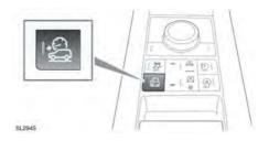
**Note:** The driver's seat belt must be buckled and all of the doors closed to enable the feature.
