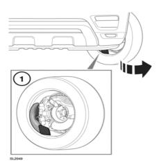
Some vehicles are fitted with brake cooling ducts at the front wheels. Pay careful attention to these areas after driving the vehicle off-road. Make sure the cooling duct (1) is clear from debris; a pressure washer may be used if required. For ease of access, start the engine and turn the steering onto the relevant full lock. Switch off the ignition.
